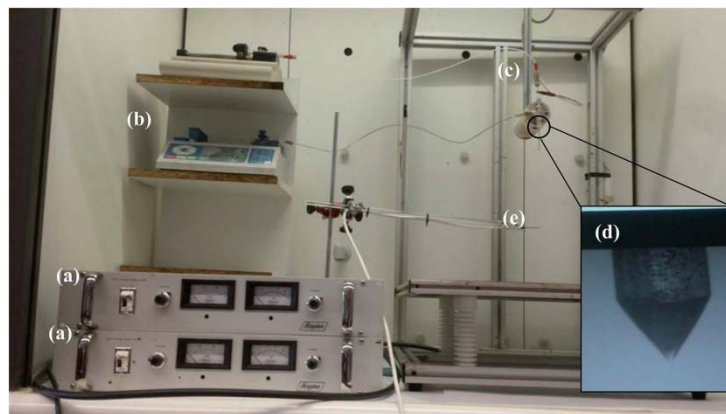
Fig.1. 電界紡糸装置. Reproduced from the above paper with permission from The Royal Society of Chemistry.
