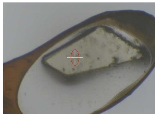
Figure 1. Unfrozen protein crystal mounted by Humid-air and glue-coating method
